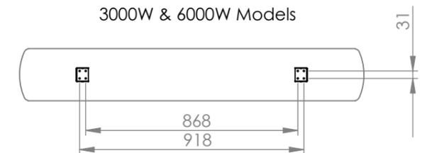
2. Heater must be installed with heater surface at least 2400mm above the floor level. Supplied suspension tubes position heater surface 1000mm below the ceiling surface. If required, cut down length of suspension tubes to ensure correct installation height. Minimum distance from front surface of heater to ceiling surface must be 250mm for 2000W & 3000W models & 330mm for 4000W & 6000W models.
