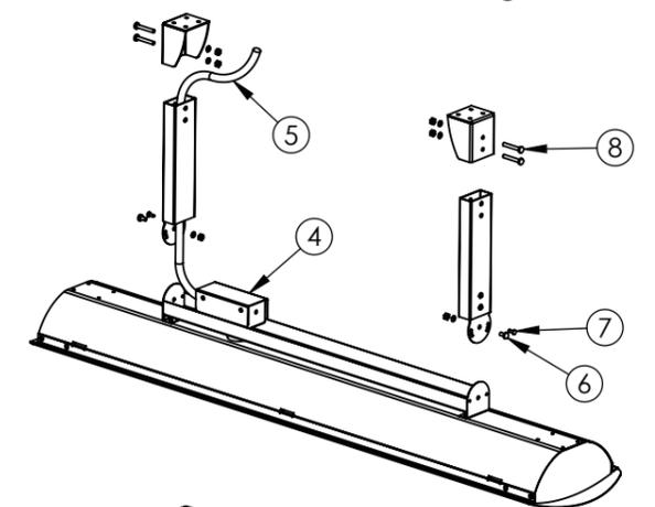
9. Make electrical connection from suspension tube power cord to power from ceiling as per electrical installation instructions in this manual.
