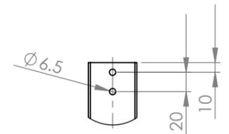
③ Suspension Tube Mounting Hole
