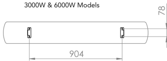
2. Attach mounting brackets to ceiling or wall using appropriate fasteners (Not supplied).
