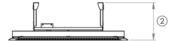
3. If suspension tubes are cut down, drill new mounting holes in each tube.
